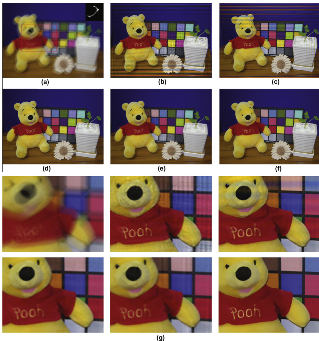
Fig. 10. Pooh. (a) Blurred image and estimated PSF. (b) Richardson–Lucy method. (c) TV regularization. (d) Levin's. (e) Shan's. (f) Proposed. (g) Close-up views of (a)–(f).
