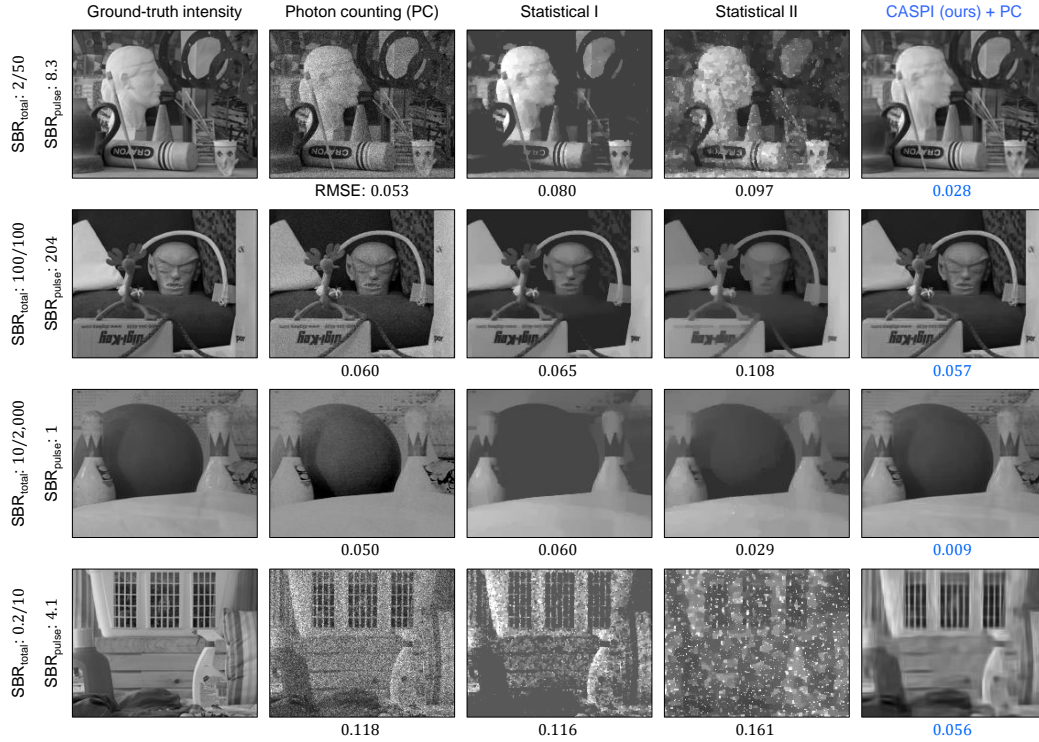
Fig. S2: Scene intensity estimation comparisons. CASPI enables high-quality scene intensity estimates by simply summing over the time dimension of the recovered photon fluxes. Compared to other approaches, our method preserves intensity details better in high signal-to-background ratio (SBR) regime ( SBR_{total} = 100/100 ) while suppressing the noise more effectively in sub-photon regime ( SBR_{total} = 0.2/10 ). In addition, the saturation and the excessive high contrast in the photon counting result are also reduced by our approach when operating in a high background flux regime ( SBR_{total} = 10/2,000 ). Root-mean-square error (RMSE) is labeled below each image as the objective performance measure.
